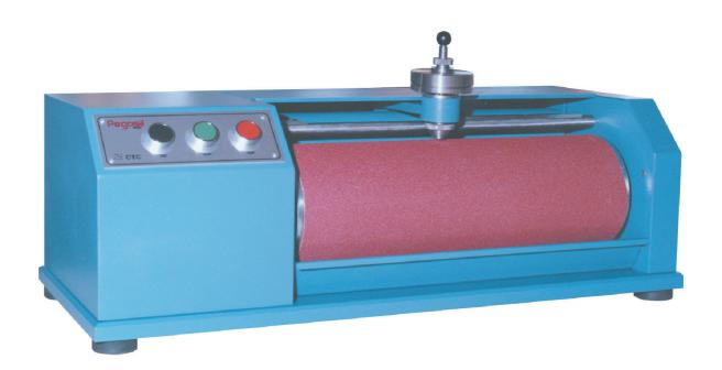
Abrasion Test Machine (type DIN) for Sole Material
